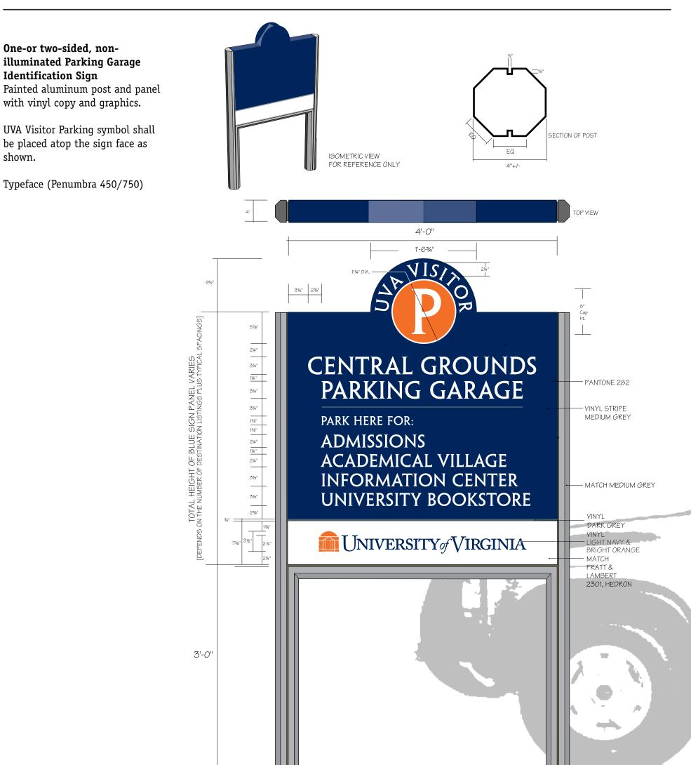
FABRICATOR NOTES: • POSTS TO BE EMBEDDED IN CONCRETE.
