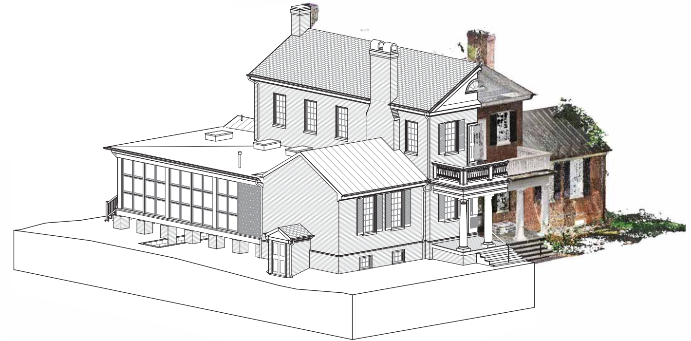
Figure 179. Point cloud image superimposed on 3D model. The measured drawings relied on laser scanning and on hand measurements. JGWA, 2024.
