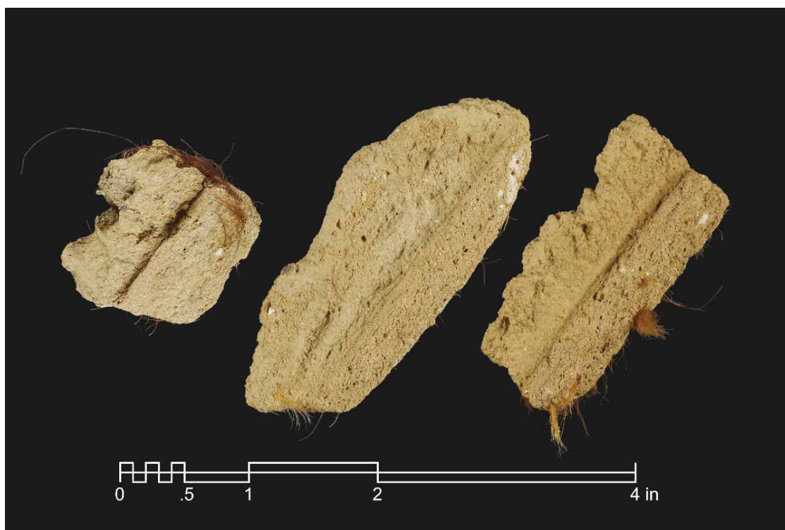
Figure 20: Lathing render tabs showing detail of hair amendments.
