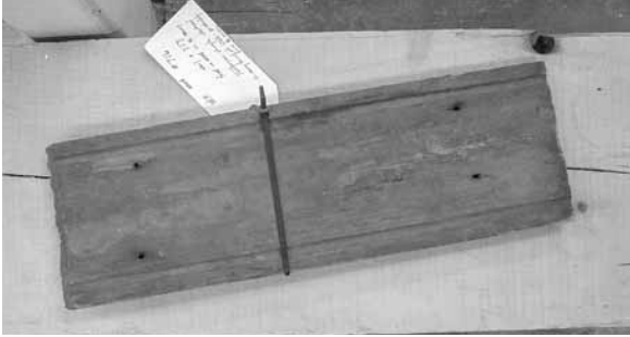
Figure 79. Shingle found in East Privy, Poplar Forest, Bedford County, Virginia, originally used on flat roof. Note grooved rainwater channels. MCWB photograph, 2004.
