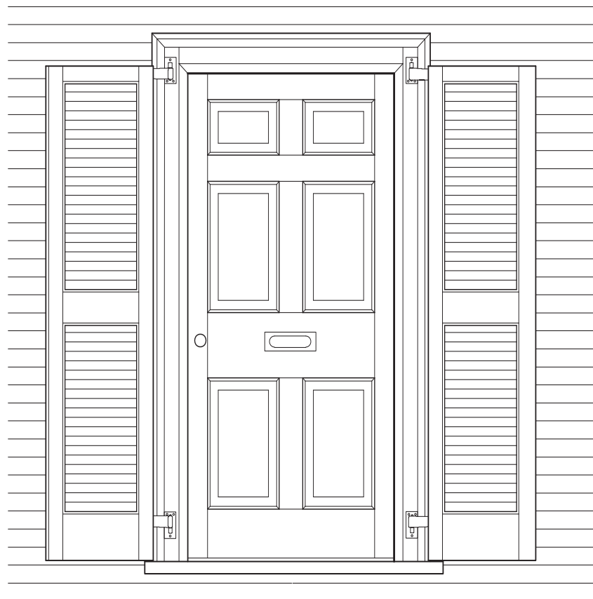
Figure 89. Elevation of surviving original door at 37 East Lawn.
