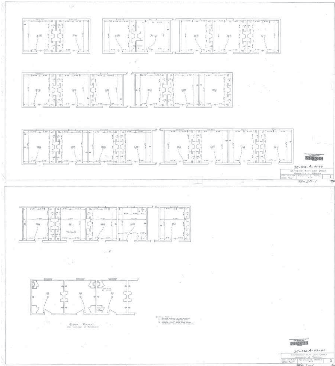
Figure 154. 1958 floor plans titled "Restoration of East Lawn Rooms" made by Frederick Doveton Nichols to illustrate then-existing conditions in East Lawn dormitories, including closets. Sheet 2, below, includes drawing of alterations for typical rooms, to include removal of closets and replacement with fixtures by the Clore furniture company. Courtesy of University of Virginia Facilities Management.
