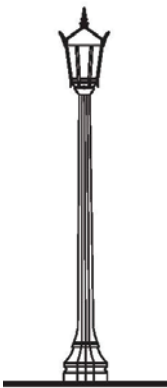
General Path Lighting, King Edgewater K-56 metal halide or LED luminaire on 12' cast aluminum or cast iron octagonal pole, Rookwood shutter green, pebbled lenses
