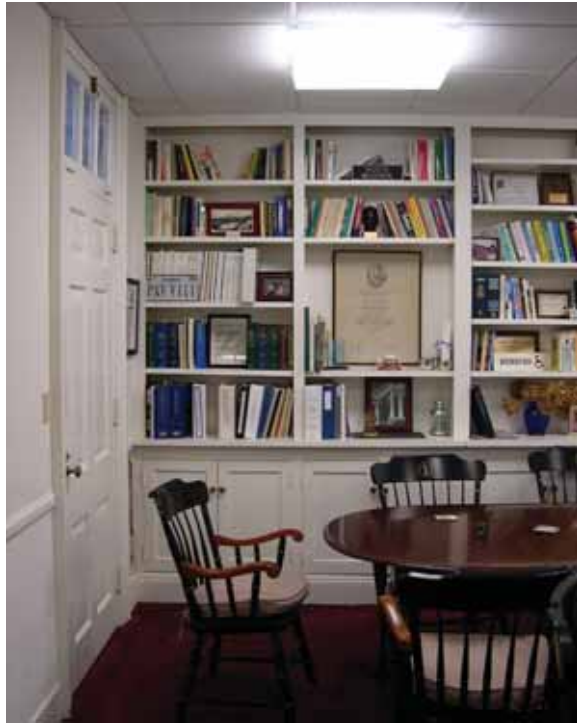
Southwest Wing, office of the Vice President for Student Affairs (124), looking west. The suspended acoustical tile ceiling and surface-mounted fluorescent light fixtures detract from the historic character of the space. The suspended ceiling obscures the upper architraves of the door/transom openings. [JGWA, 2006]
