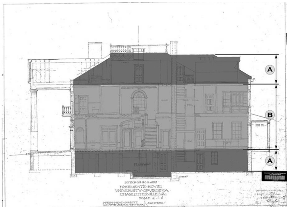
Figure S-14: Strengthening and Preservation Approach. Zone A indicates areas of significant structural intervention. Zone B indicates areas of preservation with minimal structural intervention.
