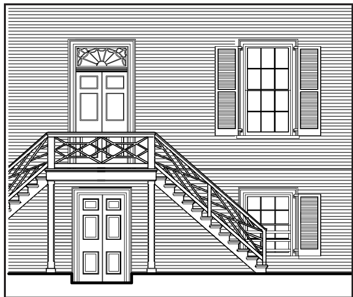
Figure 22 & 23 One set of pintles are located on the right side of the north cellar window on the east elevation. It is believed the rear stair passed in front of a portion of the cellar windows resulting in the condition illustrated above resulting in the need for only one set of pintles.
