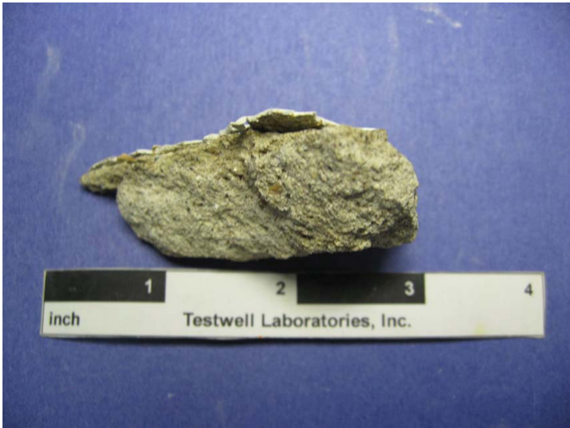
Figure 1: Render sample as received by Testwell Laboratories for mortar analysis. The sample appears homogeneous throughout with no indication of multiple campaigns. The sample is coated with several layers of a light-colored paint.
