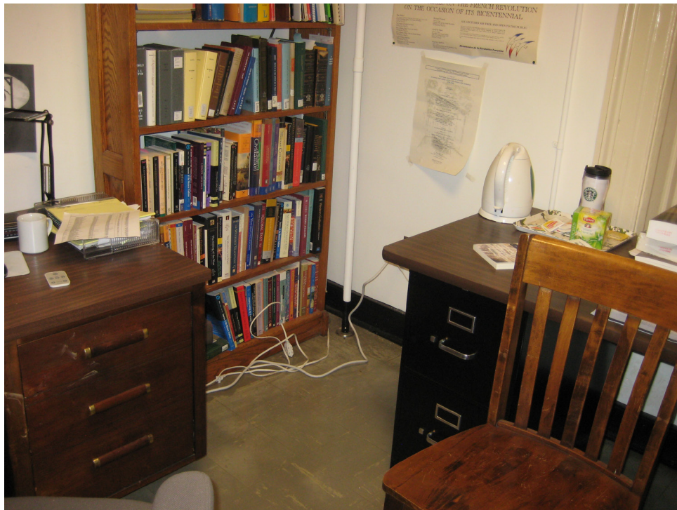
Photo 2 shows a commonly observed office scenario with a number of extension cords serving long term appliances. The electric hot beverage heater is the type of appliance that commonly is left on after work hours.
