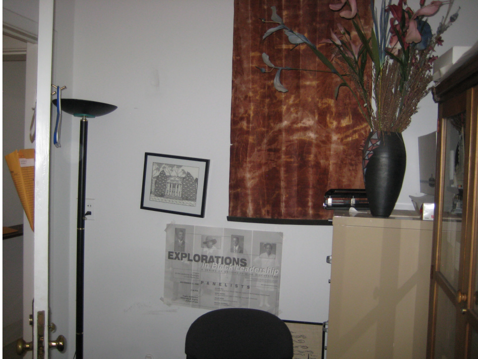
Photo 3 shows a torchiere light fixture which was observed in several offices. These lights operate at very high temperatures and are subject to materials falling on top of them. If the material is combustible (i.e. drapery) ignition can occur.
