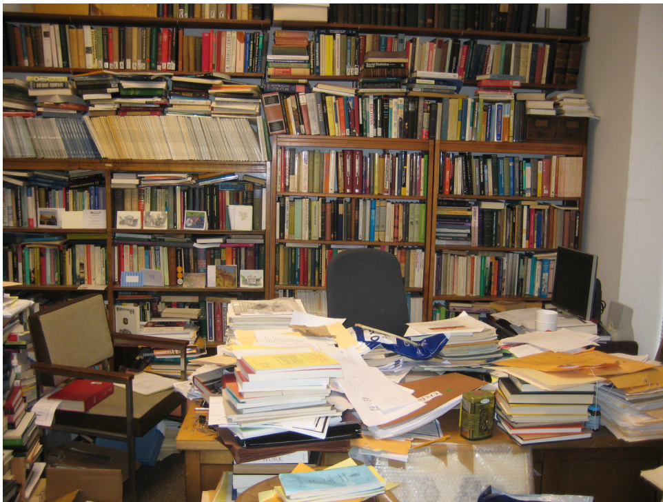
Photo 6 shows an office in Hotel F that has an extremely high fuel load. These materials are arranged so that they have a large amount of surface area and will act as a kindling type fuel. Also note the presence of the desktop computer in close proximity to fuels. Once flames have appeared this room will experience a fire that can exceed 1,200°F and ultimate flashover (full room involvement) within minutes.
